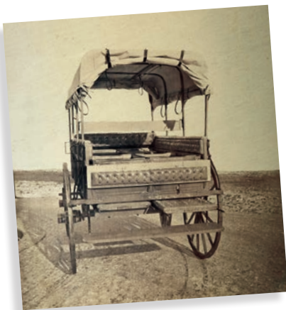
Figure 4.3 Howard Ambulance. The Howard Ambulance (from the rear) was created by Assistant Surgeon Benjamin Douglas Howard. The tailgate is partially lowered revealing the rollers that supported the cushioned litters. It was originally featured in a publication by the US Sanitary Commission. Source: New York Public Library Digital Collections. Pell, George E; circa 1861-1872.
